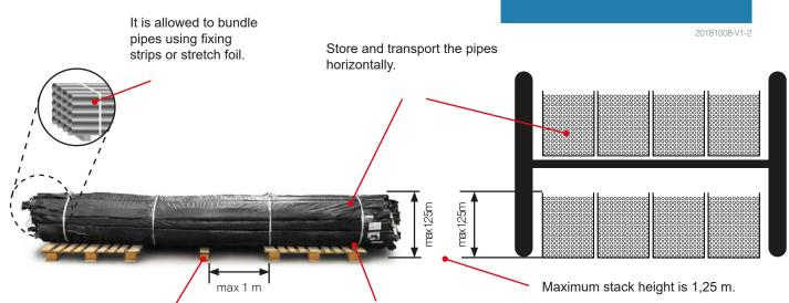
Use supports to avoid deflection. Spacing of pipes' supports shall not exceed 1 meter.
